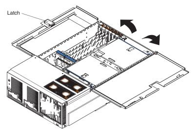
**Attention:** For proper cooling and airflow, close the cover before turning on the server. Operating the server for extended periods of time (over 15 minutes) with the cover open might damage server components.
